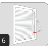
6 After charging, detach and disconnect the PowerBar, and lift it slightly and then remove it from the shade
