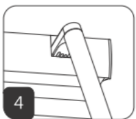
4 Align and insert the Charging Connector and the Charging port to charge the shade
